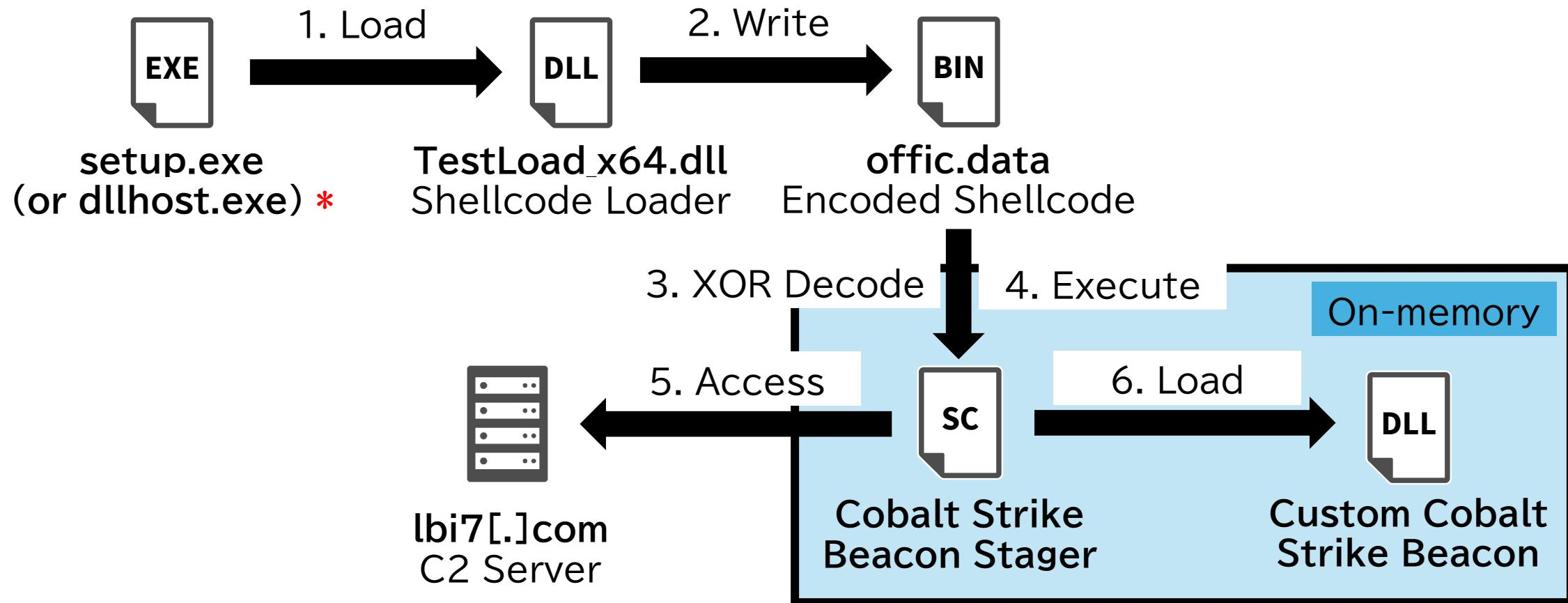
\* Loader only functions when the module filename matches the expected value.
