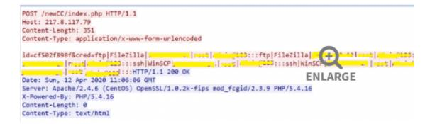
Figure 7: The POST request to send collected credentials to the C&C.
